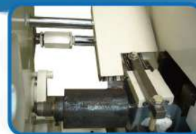
電氣射料管及鵝頸 PID加熱系統 PID ELECTRICAL NOZZLE & GOOSENECK HEATER SYSTEM
