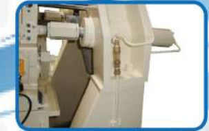
射出部冷卻流量計 INJECTION SYS. COOLING WATER FLOW INDICATOR
