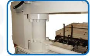
射數位化射出行程控制+ 一體成行射出缸 DIGITAL INJECTION STROKE CONTROL +ONE PIECE FRAME INJECTION CYLINDER
